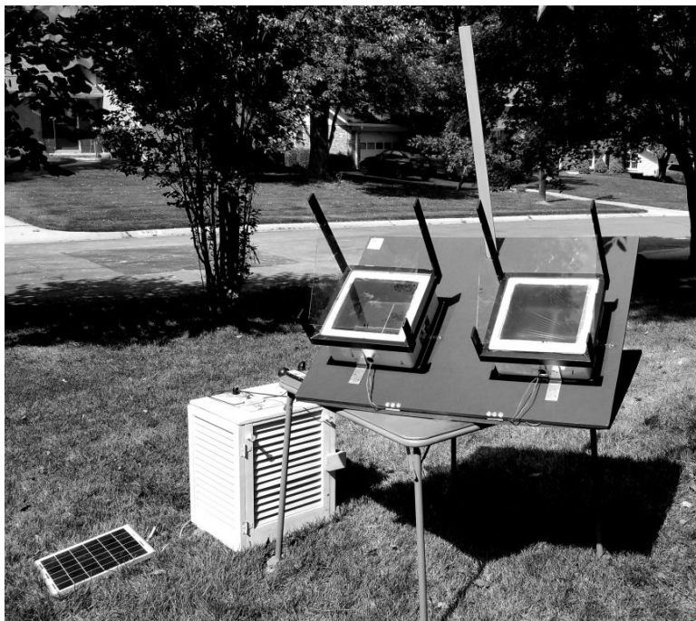
Figure 2: Experimental setup for comparison experiments. The white box is a “Stevenson box” containing weather instruments, powered by the solar panel on the ground. Each test box has a black frame holding a sheet of window glass at a 45^\circ angle. Cables from 2 cm holes in the bottom of each box are connected to thermocouples to measure internal black plate temperatures. A data logger is connected to the cables behind the tilt table.
