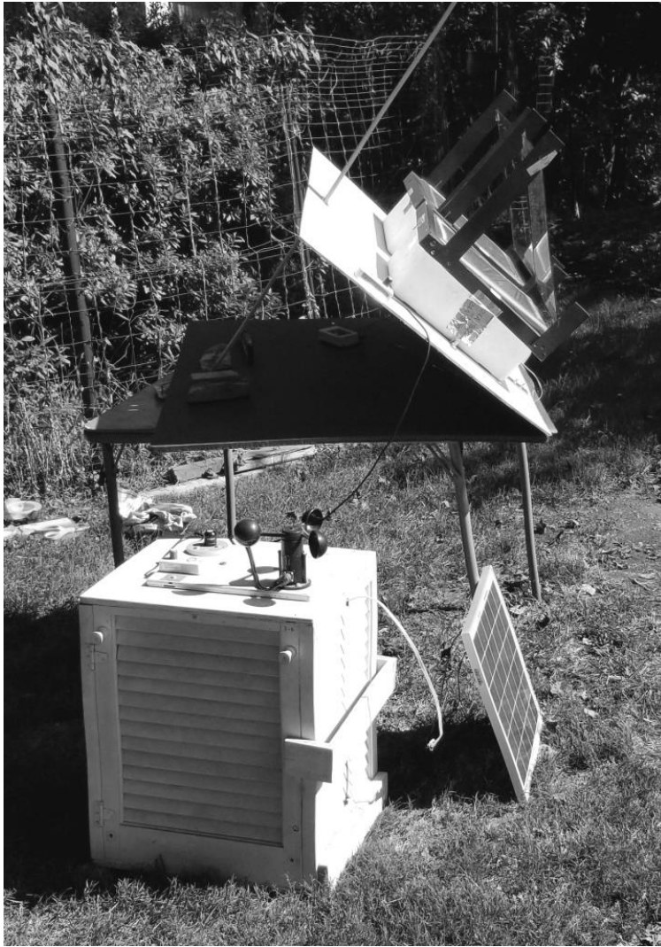
Figure 3: Side view of experimental setup showing two test boxes mounted on a tilt table to allow the boxes to be pointed in the Sun direction. Glass prefilter sheets can be seen mounted in frames in front of the boxes. There is a 4 cm air gap below the sheets to permit free convection over the boxes. A pyranometer is mounted on the tilt table for measuring global tilted irradiance (GTI), and two more are mounted on top of the Stevenson box to measure global horizontal irradiance (GHI), along with an anemometer. The Stevenson box also contains a solar panel charge converter and a data logger for storing measurements.
